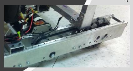
The drive motor of a robot is attached to a gear of radius 0.0320 m. A belt runs over the gear to a smaller, 0.0175 m gear attached to the front wheel, which has a radius of 0.0510 m. The robot drives at 3.00 m/s.
